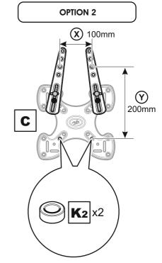
Use spacer **K2** between the bottom two holes of the bracket and your TV.
