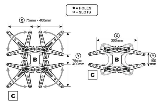
Adaptors **C** can be fixed in different positions in the slots on Plate **B** to match your TV fixing holes.
