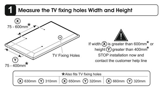
You are provided with 4 diameters of TV fixing screws, **M4**, **M5**, **M6** and **M8**. Determine the screw diameter that fits and remember for step 4.
