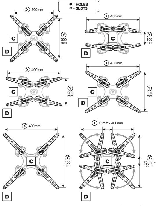
Adaptors **D** can be fixed in different positions in the slots on Plate **C** to match your TV fixing holes.
