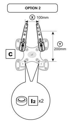
Use spacer **I2** between the bottom two holes of the bracket and your TV.
