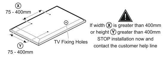
You are provided with 4 diameters of TV fixing screws, M4, M5, M6 and M8. Determine the screw diameter that fits and remember for step 4.
