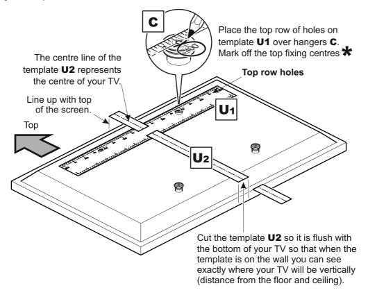
★ If hangers C do not line up with any holes on the template then ensure template is firmly in position and punch 2 holes to match your top fixing centers with a pencil or sharp object.
