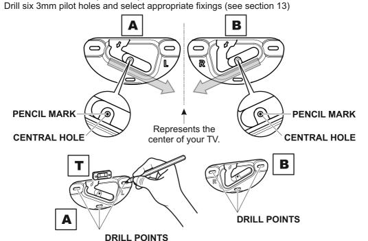
Use the correct fixings for your wall type. Mixing fixing screws may be required for installations that span different wall types. DO NOT OVER TIGHTEN SCREWS.
