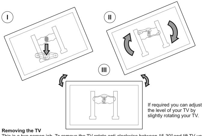
This is a two person job. To remove the TV rotate anti-clockwise between 15-30° and lift TV up and out (ie reverse the movements as shown above).
