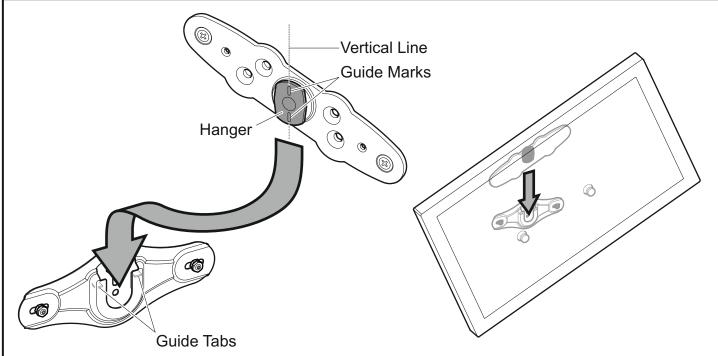
Rotate your TV so that the guide marks on the hanger are vertical. Next slide your TV down so that the hanger goes between the two guide tabs on the wall bracket. Ensure the hanger is fully engaged and rotate clockwise until your TV is level.
