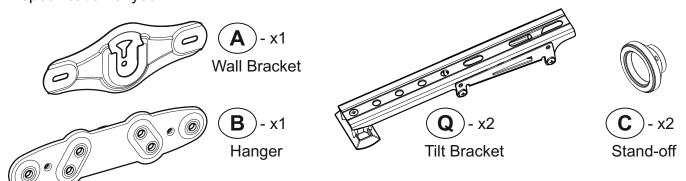
**TV Fixings:** Parts go on the back of the TV (specification of your TV will determine which ones you require - see section 9).
