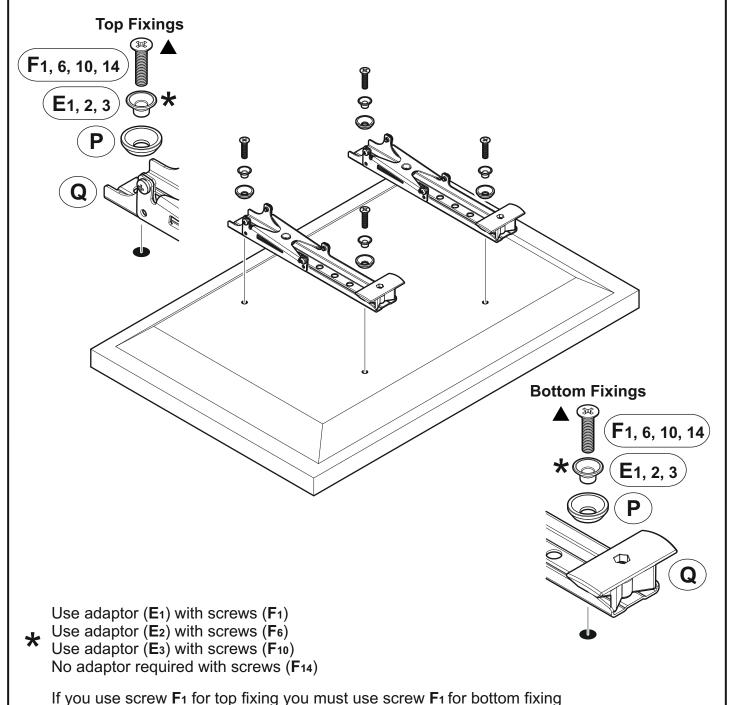
If you use screw F1 for top fixing you must use screw F1 for bottom fixing
