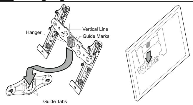
Rotate your TV so that the guide marks on the hanger are vertical. Next slide your TV down so that the hanger goes between the two guide tabs on the wall bracket. Ensure the hanger is fully engaged and rotate clockwise until your TV is level.
