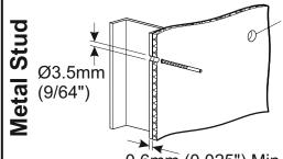
Use Plasterboard / Sheetrock fixings
