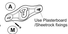
Only one fixing will be in the wood stud. The other fixings will be in plasterboard / sheetrock (see above).
