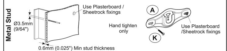
Only one fixing will be in the metal stud. The other fixings will be in plasterboard / sheetrock (see above).
