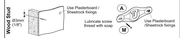
Only one fixing will be in the wood stud. The other fixings will be in plasterboard / sheetrock (see above). Lift ceiling tiles in order to ascertain location of vertical metal studs.
