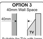
Suitable for TVs with large obstructions eg power supply, mouldings etc
