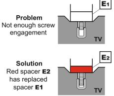
If you have a Samsung TV with Samsung Wall Mount Adapters you will have to use Screw G12. You may need to use Washer E3 to ensure Hanger C or Spacer D are fitted securely.
