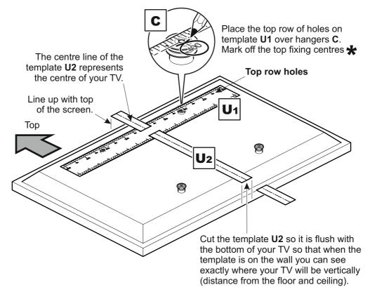
★ If hangers C do not line up with any holes on the template then ensure template is firmly in position and punch 2 holes to match your top fixing centres with a pencil or sharp object.
