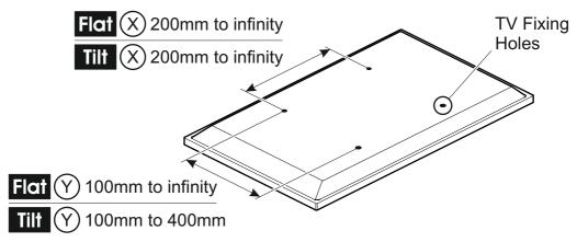
If width (X) is less than 200mm or height (Y) is less than 100mm STOP installation now and contact the customer help line
