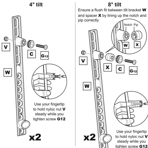
Ensure a flush fit between tilt bracket W and spacer X by lining up the notch and Notch Pip Use your fingertip to hold nyloc nut V steady while you
