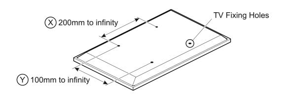
If width (X) is less than 200mm or height (Y) is less than 100mm STOP installation now and contact the customer help line
