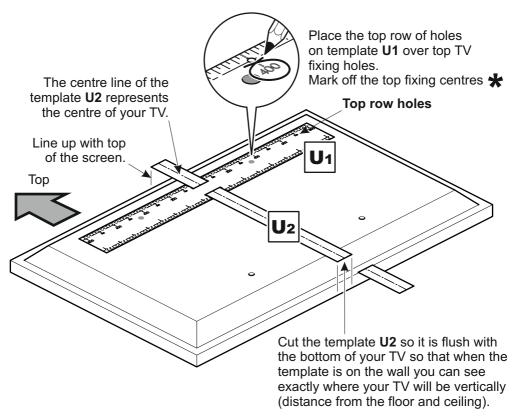
If top TV fixing holes do not line up with any holes on the template then ensure template is firmly in position and punch 2 holes to match your top fixing centres with a pencil or sharp object.
