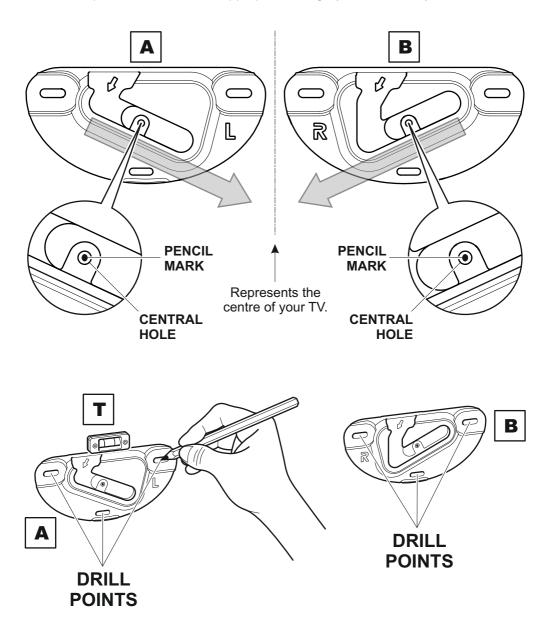
Use the correct fixings for your wall type. Mixing fixing screws may be required for installations that span different wall types. DO NOT OVER TIGHTEN SCREWS.
