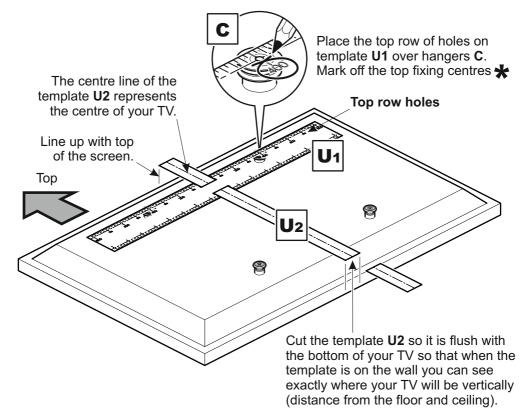
★ If hangers C do not line up with any holes on the template then ensure template is firmly in position and punch 2 holes to match your top fixing centres with a pencil or sharp object.
