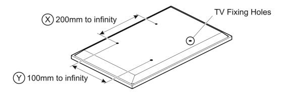
If width  $\bigotimes$  is less than 200mm or height  $\bigotimes$  is less than 100mm STOP installation now and contact the customer help line
