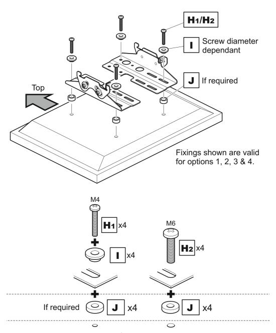
Attach the bracket to the back of your TV using suitable screw, reducer and spacer combinations.
