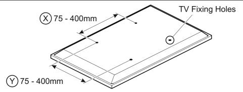
If width (X) is greater than 400mm or height (Y) greater than 400mm STOP installation now and contact the customer help line
