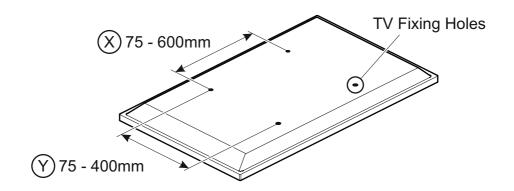
If width (X) is greater than 600mm or height (Y) greater than 400mm STOP installation now and contact the customer help line
