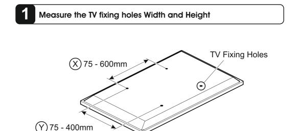
If width  $\bigotimes$  is greater than 600mm or height  $\bigotimes$  greater than 400mm STOP installation now and contact the customer help line
