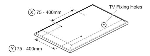
If width (X) is greater than 400mm or height (Y) greater than 400mm STOP installation now and contact the customer help line
