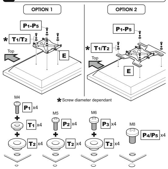
Attach the bracket to the back of your TV using suitable screw, and reducer combinations.
