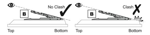
If a clash is observed you will need to use adaptors **C** to position the TV Brackets **B** closer to the bottom of the TV to achieve maximum tilt.
