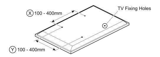
If width (X) is greater than 400mm or height (Y) greater than 400mm STOP installation now and contact the customer help line
