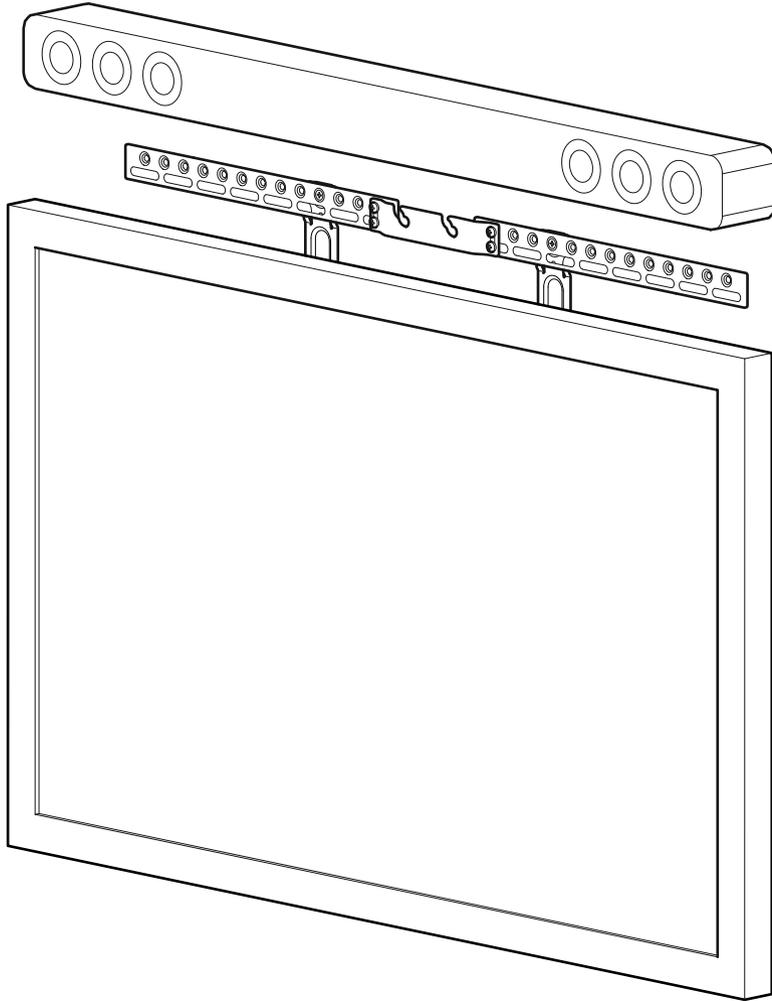
**7****Attaching to Soundbar with Keyhole Pin****Montage du Soundbar au moyen des attaches pour trou de serrure**
