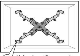
Holes do not line up and small adjustment is required before you fully tighten
