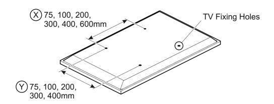
If width (X) is not equal to 75, 100, 200, 300, 400 or 600mm or height (Y) is not equal to 75, 100, 200, 300, 400mm STOP installation now and contact the customer help line
