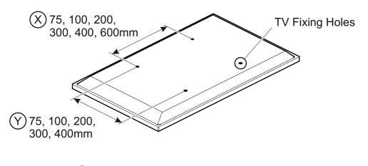
If width  $\bigotimes$  is not equal to 75, 100, 200, 300, 400 or 600mm or height  $\bigotimes$  is not equal to 75, 100, 200, 300, 400mm STOP installation now and contact the customer help line
