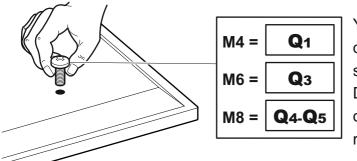
You are provided with 3 diameters of TV fixing screws, **M4**, **M6** and **M8**. Determine the screw diameter that fits and remember for step 3.
