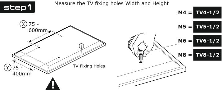
If width (X) is greater than 600mm or height (Y) greater than 400mm STOP installation now and contact the customer help line
