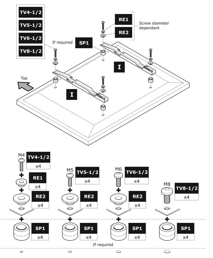
Attach the bracket to the back of your TV using suitable screw, reducer and spacer combinations. If you have any issues fitting to the back of your TV with the supplied screws, please call the customer services helpline.
