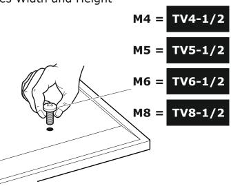
You are provided with 4 diameters of TV fixing screws, **M4**, **M5**, **M6** and **M8**. Determine the screw diameter that fits and remember for step 10.
