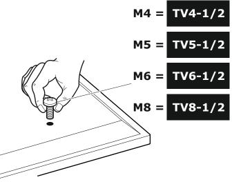
You are provided with 4 diameters of TV fixing screws, **M4**, **M5**, **M6** and **M8**. Determine the screw diameter that fits and remember for step 10.
