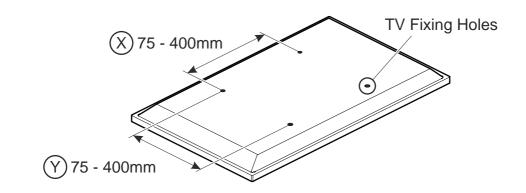
If width  $\bigotimes$  is greater than 400mm or height  $\bigotimes$  greater than 400mm STOP installation now and contact the customer help line
