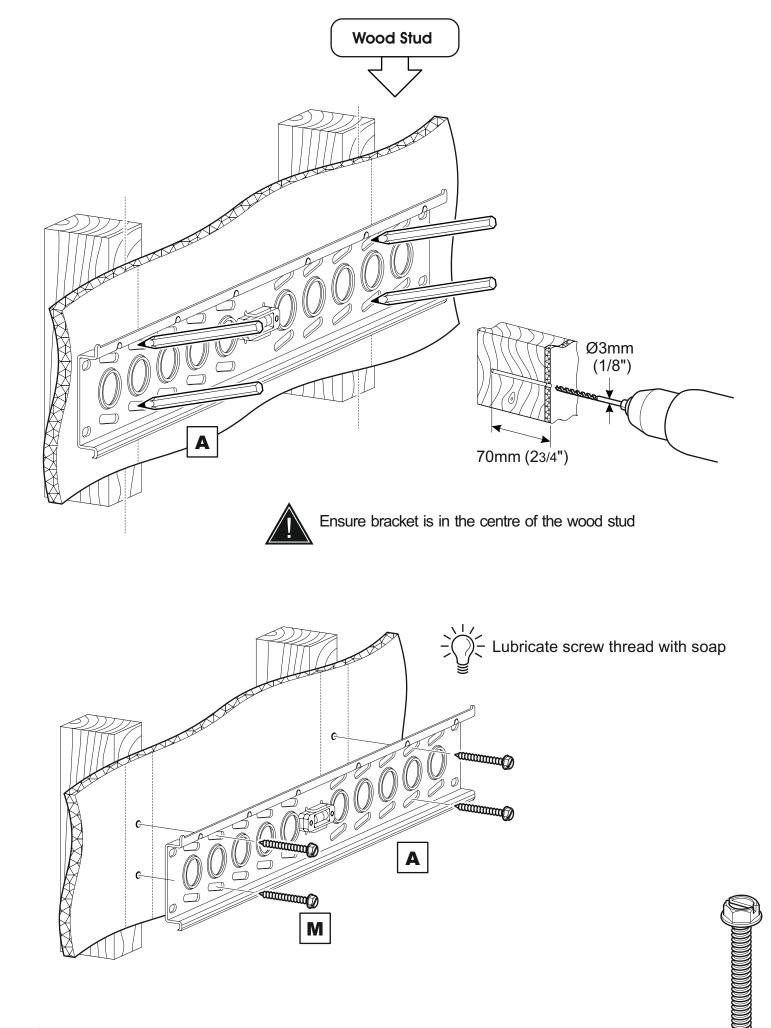
Ensure level before final tightening. DO NOT over tighten screws. Tighten screws by hand only 1. Hang Shelf Bracket
