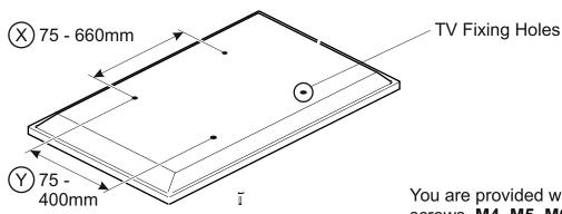
You are provided with 4 diameters of TV fixing screws, M4, M5, M6 and M8. Determine the
