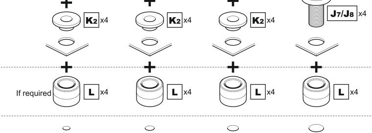
Attach the brackets to the back of your TV using suitable screw, reducer and spacer combinations
