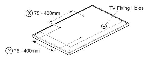
If width X is greater than 400mm or height Y greater than 400mm STOP installation now and contact the customer help line
