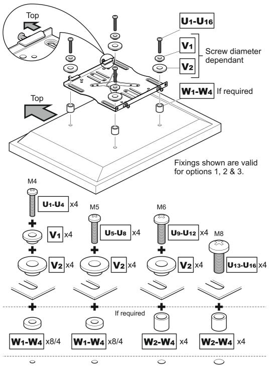
Attach the brackets to the back of your TV using suitable screw, reducer and spacer combinations.
