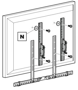
The brackets and the screws shown in grey are only an example. These are supplied by the TV wall mount manufacturer.
