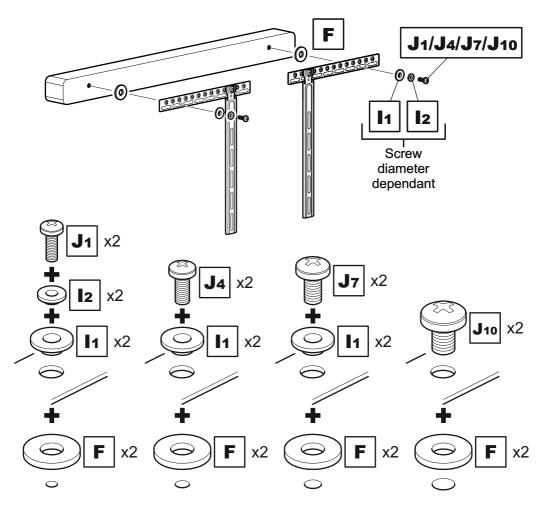
Attach the brackets to the back of your TV using suitable screw and reducer combinations.
