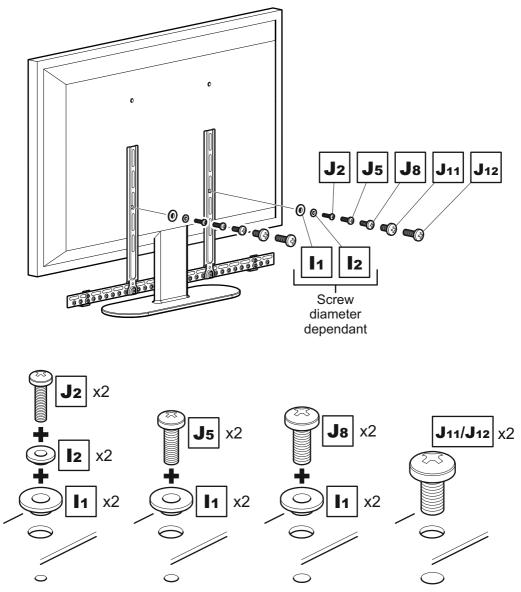
Attach the brackets to the back of your TV using suitable screw and reducer combinations.
