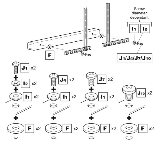
Attach the brackets to the back of your TV using suitable screw and reducer combinations.
