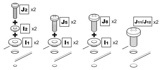
Attach the brackets to the back of your TV using suitable screw and reducer combinations.
