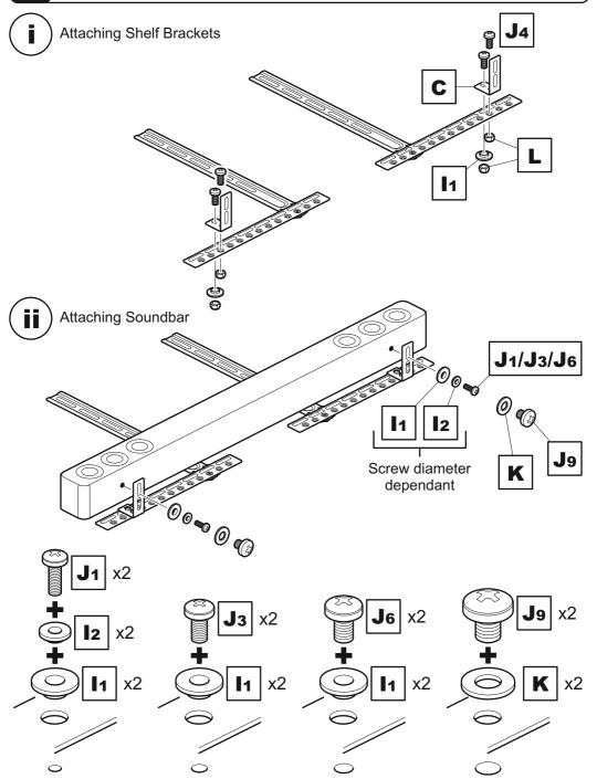
Attach the brackets to the back of your TV using suitable screw and reducer combinations.
