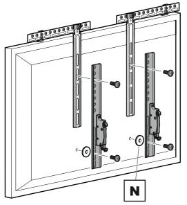
The brackets and the screws shown in grey are only an example. These are supplied by the TV wall mount manufacturer.
