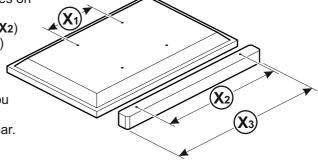
Before you attach horizontal bracket **B** to vertical bracket **A** use measurements **X1** and **X2** or **X1** and **X3** to decide the best configuration. Please see below for examples.
