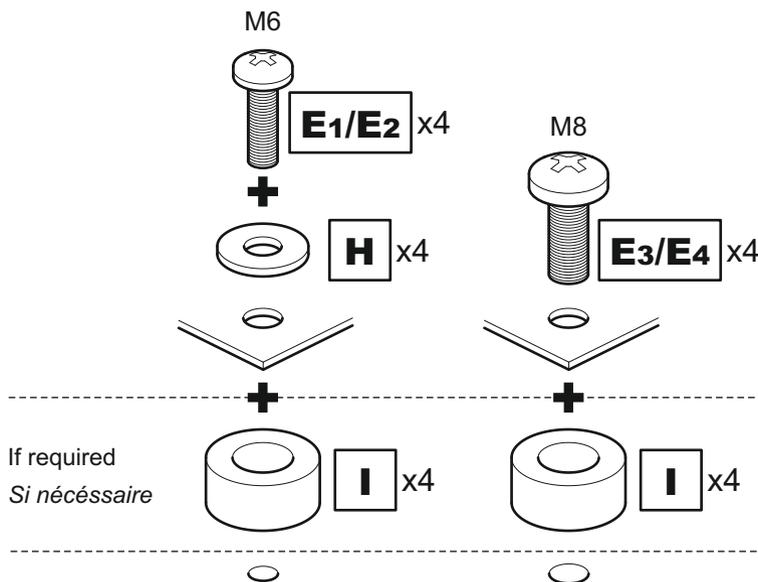
Attach the bracket to the back of your TV using suitable screw, reducer and spacer combinations.
