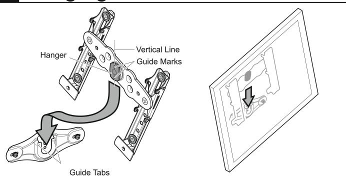
Rotate your TV so that the guide marks on the hanger are vertical. Next slide your TV down so that the hanger goes between the two guide tabs on the wall bracket. Ensure the hanger is fully engaged and rotate clockwise until your TV is level.
