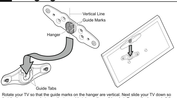
that the hanger goes between the two guide tabs on the wall bracket. Ensure the hanger is fully engaged and rotate clockwise until your TV is level.
