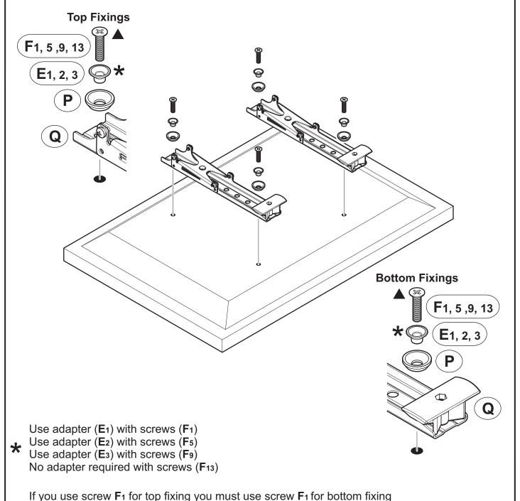
If you use screw F<sub>1</sub> for top fixing you must use screw F<sub>2</sub> for bottom fixing
