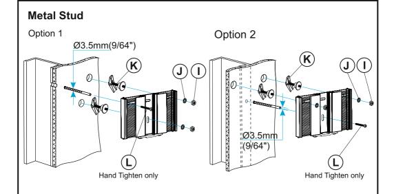
Only one fixing will be in the metal stud. The other fixings will be in plasterboard/ sheetrock.
