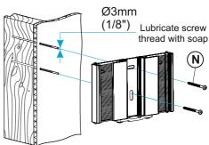
Only one fixing will be in the wood stud. The other fixings will be in plasterboard/ sheetrock(see above).
