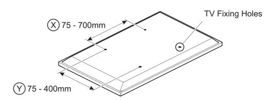
If width (X) is greater than 700mm or height (Y) greater than 400mm STOP installation now and contact the customer help line
