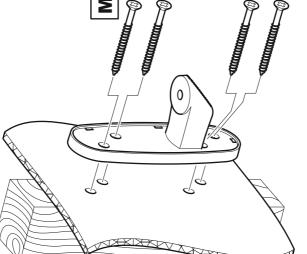
DO NOT over tighten screws Tighten screws by hand only
