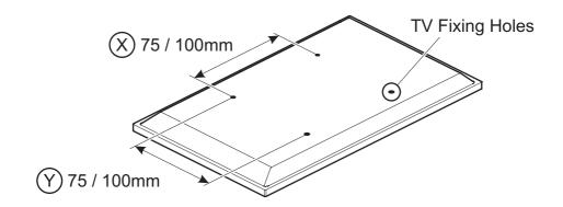
If  $\bigotimes$  or  $\bigotimes$  are not equal to 75 or 100mm STOP installation now and contact the customer help line.
