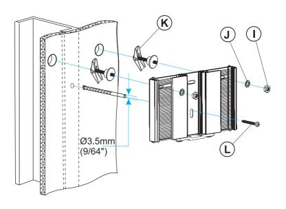
Only one fixing will be in the metal stud. The other fixings will be in plasterboard/ sheetrock.
