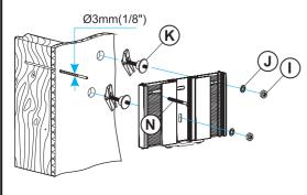
Only one fixing will be in the wood stud. The other fixings will be in plasterboarrd/ sheetrock(see above). Option 2
