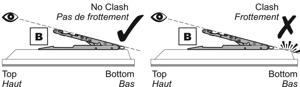
If a clash is observed you will need to use adaptors **C** to position the TV Brackets **B** closer to the bottom of the TV to achieve maximum tilt.
