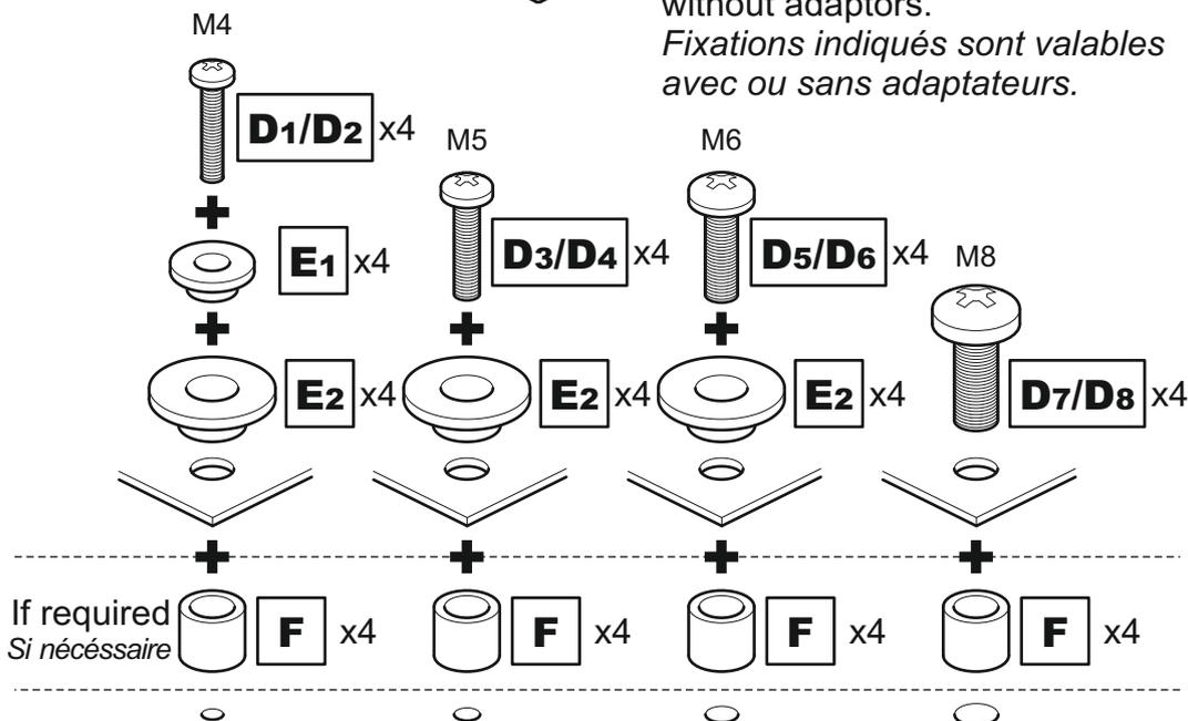
Attach the bracket to the back of your TV using suitable screw, reducer and spacer combinations.
