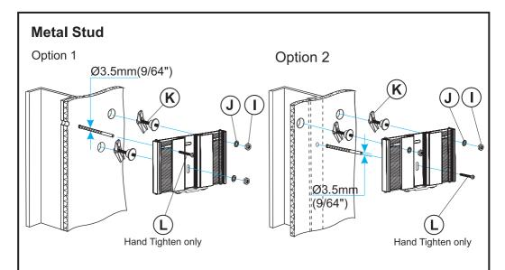
Only one fixing will be in the metal stud. The other fixings will be in plasterboard/ sheetrock.
