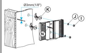
Only one fixing will be in the wood stud. The other fixings will be in plasterboard/ sheetrock(see above).
