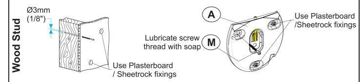
Only one fixing will be in the wood stud. The other fixings will be in plasterboard / sheetrock (see above).
